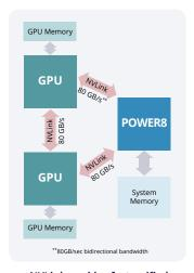
NVLink enables fast unified memory access between CPU and GPU Memories
