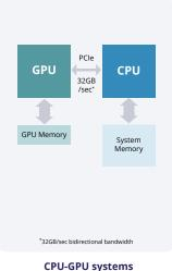
CPU-GPU systems connected via PCI-e
